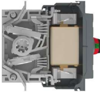
Pole structure in OFF- position
